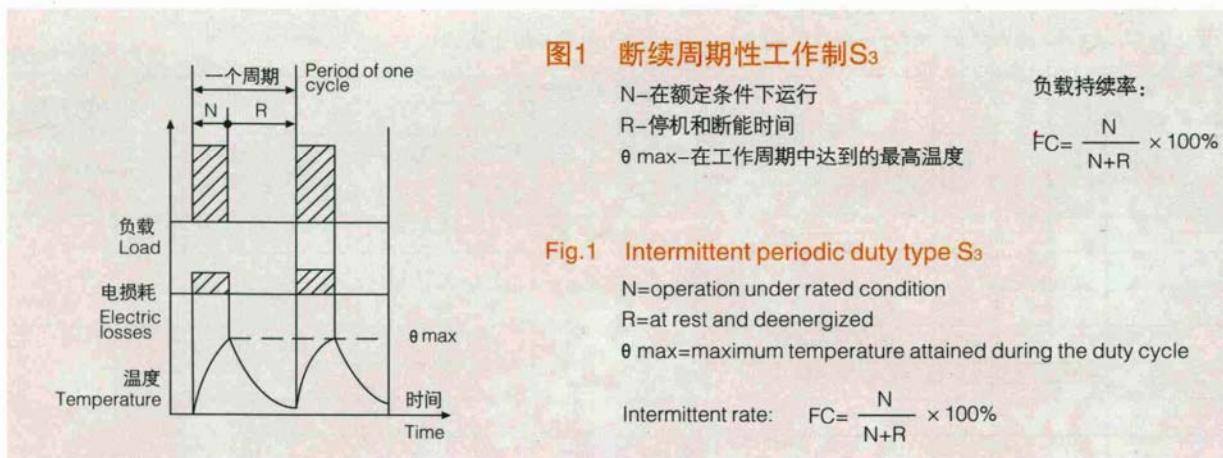
Fig.1 Intermittent periodic duty type S<sub>3</sub>
